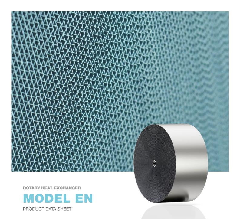
Model EN is a high-performing small rotary heat exchanger without casing, designed to be fitted directly inside an air handling unit or mounted in a cassette, primarily for residential ventilation applications. Typical temperature efficiencies are between 75-80%, but with design optimization, the efficiency can approach 90%.
