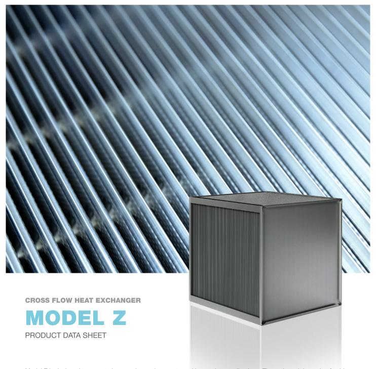
Model Z is designed to operate in corrosive environments and heavy duty applications. The entire unit is made of acid resistant stainless steel and a single pass exchanger can provide a sensible efficiency of 65 - 70%.
