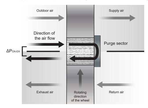
"The purge sector is a device that can practically prevent air leakage resulting from the rotation of the wheel (*carryover*)" - REHVA, Limiting internal air leakage across the rotary heat exchanger.
