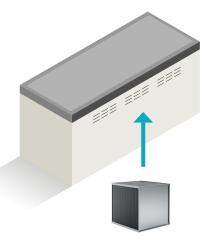
The heat exchanger is usually located in the top part of the inverter cabinet.
