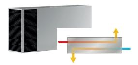
Two airstreams flow in opposite direction to one another. The airflow in our counter flow heat exchangers can be adjusted in several different ways.
