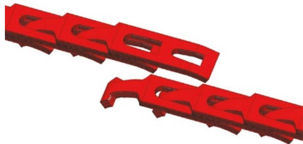
Figure 36. Remove excess belt to obtain good tension.
